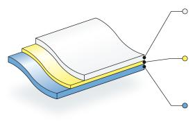
**Facestock:** 2 mil optically clear polyester that offers excellent clarity and dimensional stability combined with good high temperature and humidity resistance. The optically clear polyester provides high resolution imaging with excellent adhesion to UV curable inks.
